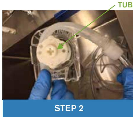
Flip the Pump Cap upside down (as pictured above) and unthread the tubing from the Tube Rotor.
