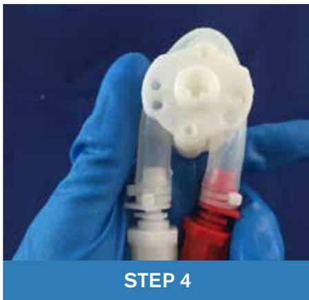
Thread your new tube set around the Tube Rotor (as pictured above). It is important that the red tube component is on the right side in this step.
