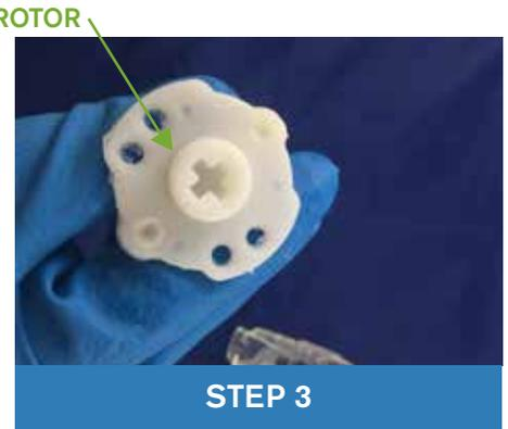
Now that the old set has been taken out, remove the Tube Rotor from the Pump Cap.
